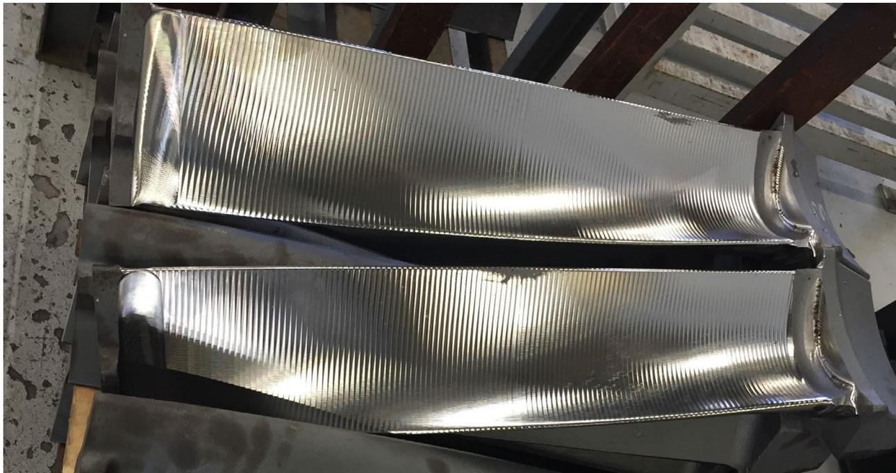
Machining was performed using the MaxiMill A251.50.R.05-12-RS.
