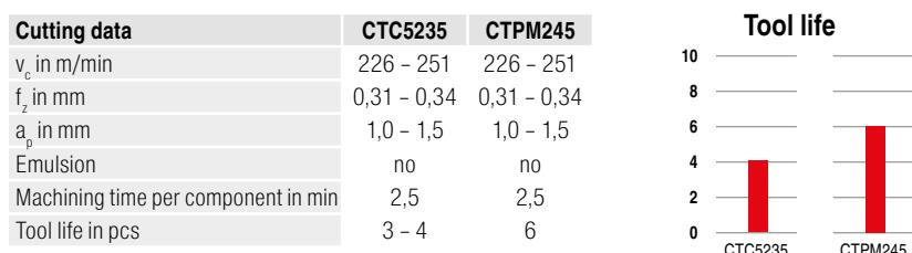
Tool life increases from 3 – 4 to a consistent 6 pcs with the same cutting parameters.
