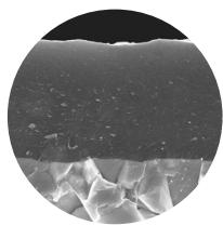
**Specifications:**Composition: Co 10.0%; other 1.5%; rest TC | Grain size: coarse | Hardness: HV<sub>30</sub> 1330 |
