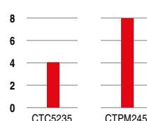
**Machining time was reduced by up to 11% and the tool life was doubled.**
